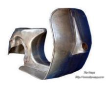
As a matter of course we replace the floor plans on all our vespas with a thicker grade of steel, these floor pans are imported from India and come off the original Piaggio presses. Once all traces of rust have been removed, Any dents or imperfections are beaten out this often as long as 2 days! Unlike other restoration companies we avoid using excessive body filler! The next stage is to put the scooter on a jig to check for 100% trueness.
