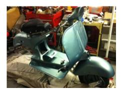
The handlebars were then set in place before the very tricky task of installing the new cables, carefully routing through the frame: July 2011, things are a little on hold due to an ankle injury, however I will use this time to try and source a few other new bits that are required:
