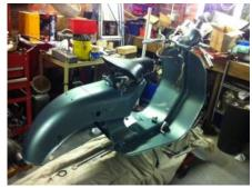
While the frame was being painted, I refurbished and painted the front fork assembly, so on return of the frame, the first task was to fit the forks, mudguard and new steering bearings. The original stand was also fitted with new rubber feet and fitted to make the rest of the assembly a little easier
