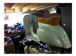
For the purists out there, this scooter had already been modified, had an ACMA style rear end and seat, with exposed cables, chrome headset/handlebar assembly etc. First thing was to dump the old engine, convert back to concealed cables and fit the new handlebar assembly.
