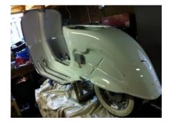
Seat posts were cut off and welded back up to accept a GS150 seat...
