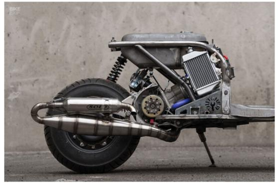
To compensate for the bigger and stronger powertrain, Butcher Garage replaced the Vyatka's bolt-on subframe with a new, reinforced unit. It's flanked by a pair of radiators, each equipped with a fan for extra cooling. An upgraded Bitubo shock props up the tail.
