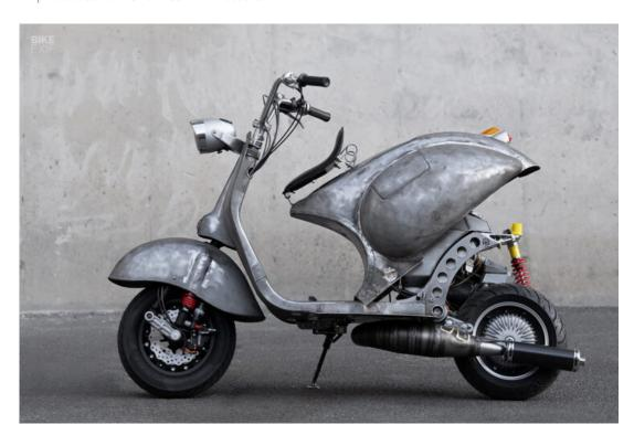
They hacked the entire rear section of the body off, before welding the wheel wells and service hatch directly to the main piece and filling in the gap left by the original seat pan. The whole thing was then re-mounted on a hinge, turning it into one giant cover for the motor. It's accessed via the main ignition key and lifts on a hydraulic strut.
