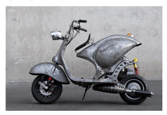
They hacked the entire rear section of the body off, before welding the wheel wells and service hatch directly to the main piece and filling in the gap left by the original seat pan. The whole thing was then re-mounted on a hinge, turning it into one giant cover for the motor. It's accessed via the main ignition key and lifts on a hydraulic strut.
