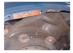
Now we take off the downpipe. You'll need an open ended spanner for the clutch side, but you can use a socket on the flywheel side. (you can also see the hole where the shroud bolts on this side
