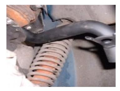
Replace the engine shroud. If you haven't already done it, replace the crossmember bolt. Now replace the rear wheelrim.
