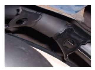
I found the best way to attach the spring to the downpipe was to use a loop of string to pull it down and through the hook on the expansion box, then the string can be untied or cut. Keep a loop in your traveling toolkit just for this purpose.
