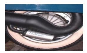
There we are, all done. It's a damn sight louder than the original part, but seems to produce a little bit more power on acceleration, perhaps losing some top end. I have been informed that when mated with a properly ported Polini 130cc kit it really shines. Being a clone of the Polini pipe that doesn't surprise me.
