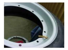
Step 5 Set the rim into the tire noting that the filler tube points toward the opposite side as shown. Align the filler hole in the rim with the mark you found earlier.
