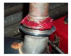
The only problem with using the existing 8" race is that some have free bearings which can be a pain to install. To make things easier, grease up the bearing race to stick the ball bearings in place. Use as much grease as you like as it will all be pushed out when the forks are installed.
