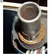
Fit the lock washer and make sure the tab is in the groove. Refit the final nut and tighten down with the same method used before on the lower nut. Finally, refit the headset by flipping it over and installing and tightening the main pinch bolt. Be sure to use a lock nut on the pinch bolt as you don't want it to ever get loose. Align the headset and the mudguard by looking down from above before the pinch bolt is tightened all the way.
