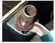
Remove the and tight upper steering fork nut and grease up the caged upper bearing race to install it in the channel. Tighten the lower race nut by hand (the one with a groove in the bottom surface) and then tighten it with the special tool, a set of vise-grips, or a hammer and screw driver.
