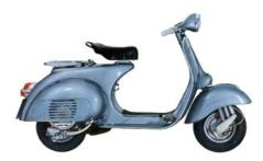
The original 1960 VBB were fitted with 8" wheels and small brakes and as a consequence did not handle as well as the large frame Vespa's with 10" wheels. Don't fear you can upgrade your VBB to fit 10" wheels. This is what you will need to do;
