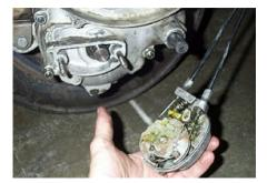
All the crankcase bolts can now be released. Both the flywheel and stator plate must be removed to get to the crankcase bolts around the main crank. Click here for the flywheel removal page.
