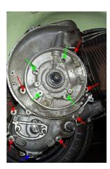
This should be the moment of truth. Refit the kick start and tighten it down - it makes a handy thing to pull on. I usually start by placing one hand behind the flywheel air scoop just below the carb box, and the other on the kick start. You shouldn't have to pull very hard to get things moving and once the casing has cleared the crankshaft it can be removed completely.
