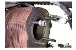
Then take either two 13mm wrenches or a single 13mm wrench and a 13mm socket (as shown below) and tighten the nuts against each other
