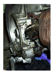
You may find that a single spring and a kickstart gear will fall out of the engine when the casings are split and this is completely normal. Once we put this back together again I'll post a page showing where they are supposed to go. Now the casings should be apart and you are ready to replace bearings, replace the shift cross or gears, fit a new casing gasket, replace the kick start rubbers, etc..
