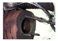
Once both flywheel side casing studs have been removed the barrel must slide up about 1/4 of an inch to allow a small locating stud in the barrel to dislocate from the casing as shown below with the red arrow - This picture was taken before the barrel studs were removed (by mistake) and the barrel stud is shown with the green arrow to avoid confusion.
