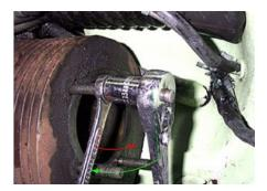
Once tight, loosen the upper nut and the stud should turn and unscrew from the casing. Leave the two nuts on the stud as they can be
