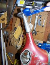
So I worked it back and forth like that with the pipe wrench till it was moving a little more freely, then forced a screwdriver gently under the flange that holds the clutch lever to pry it up, and was able to get it to start extracting. Once I got it out about 1/2 inch, then I was able to grab the tube by hand (using a rag to keep from burning my hand -- it was still hot) and pull it all the way out.
