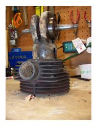
This thing must have had a pool of water inside of it for 20 years. The entire top end was one solid rusted piece of metal. Piston, cylinder, bearings, flywheel. One piece now! I'll post a picture below, it really is pretty impressive. SO now I needed to add a new top end and flywheel to the list of parts to get.
