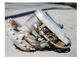
Now that the front fork is totally off, I can rebuild it. Which will have to wait for a future weekend. But here's a picture so I remember where all the cables go so I can get it back together again... Note that the brake cable goes up inside the end of the tube, while the speedometer cable comes up alongside the spring and into a hole in the tube further up (but before the bend).
