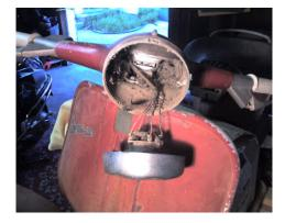
Looking inside the headset was amazing -- talk about cobwebs and dirt! How did that all get in there? Oh well. Time to remove the headset, by unscrewing the center screw on bottow, allowing the speedometer to be pushed up. Undo the "gland nut" (What the?) and remove the speedometer. Then unattach the brake cable.
