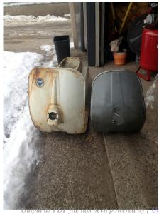
On the left is the original frame. On the right is the SS90 legshield from Scooter Center Klon in Germany
