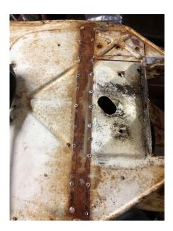
The support has been removed. Vespa didn't paint or prime before the support was attached so it was very rusty.
