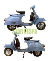
Details: Similar to the Sprint, but 8 inch wheels and smaller panels/fender/headset. Small speedo. Often has a bench seat.
