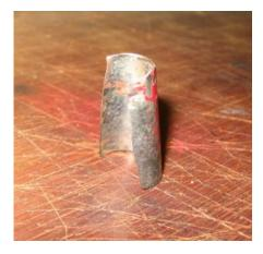
This piece of beer can was found around the crankshaft of a VBB Vespa to fill the space between the Flywheel and the Shaft
