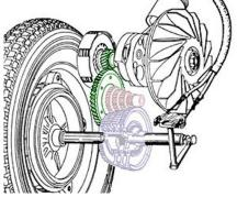
The output shaft gears are independently machined but should always go in as a group. This is the final drive, and a small machined cross locks each gear rotation independently to the output shaft rotation which is rigidly attached to the rear wheel. So all the gears spin when the bike is moving, by rotating freely on the output shaft, but only one gear at a time drives the shaft. The metal cross is moved up and down the output shaft by the gear twist grip on the handlebars.
