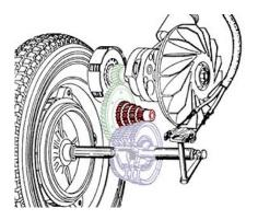
**The Primary Drive** - A small gear is attached to the drive plate of the clutch and it mates with a helical cut gear which is riveted to the input shaft. These rivets can be drilled out to change the primary drive but usually the small clutch gear must also be changed. **The Input Shaft**- This has the 3 or 4 gears machined into a single piece sometimes called a 'Christmas Tree'. The kickstart gear turns on the end of this shaft.
