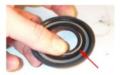
To remove the clutch side seal use a screw driver to poke it out through the main bearing. Fitting a new one is as easy as pushing it in to place. The main oil seal is made from rubber with a metal center and has a circular spring around a flexible lip. This spring must always face the pressure (i.e. the crank web). Above is a shot illustrating the ring (arrowed) with the rubber lip peeled back.
