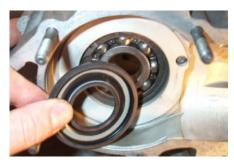
Above is the correct orientation of the clutch side oil seal. You can see the main bearing and circlip beyond. Older Vespas are similar except that the oil seal is outside the main bearing instead of inside. The difference is that when the bearing is on the crank side of the seal it is lubricated by the two stroke oil/gasoline mix, and when the bearing is on the outside of the oil seal it is lubricated by the transmission oil
