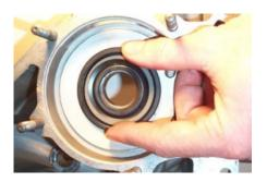
Place the oil seal in with your fingers and push hard around the edges. Try to get the outer lip flush with the casing. This isn't always possible and when it is stubborn you can use a large washer as long as the outer diameter of the washer is larger than the diameter of the seal. Use a hammer and tap the face of the washer until the washer is flush with the casing.
