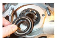
Above is the correct orientation of the clutch side oil seal. You can see the main bearing and circlip beyond. Older Vespas are similar except that the oil seal is outside the main bearing instead of inside. The difference is that when the bearing is on the crank side of the seal it is lubricated by the two stroke oil/gasoline mix, and when the bearing is on the outside of the oil seal it is lubricated by the transmission oil
